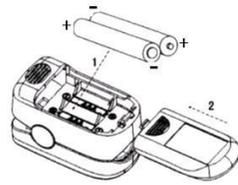
Notes: Battery polarities must be correctly installed. Otherwise, damage might be caused to device.
